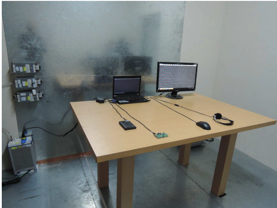
Photograph 6: Set-up for for Mains Conducted testing Front
