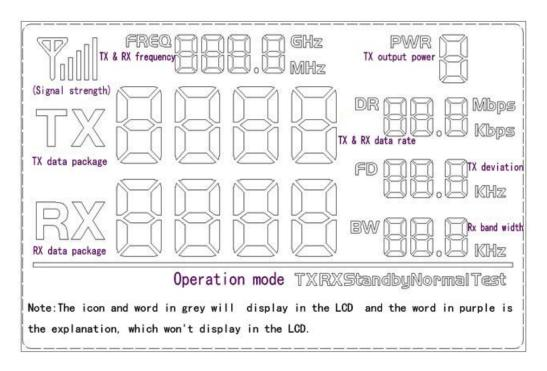
Users can set the parameters of the RF module such as frequency / transmitter power / transmission data rate / working mode through the buttons, and measure the wireless communication distance. Also, all the connection Pins of the module are extended to the demo
