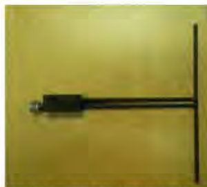
Figure 1 – MVG COMOSAR Validation Dipole
