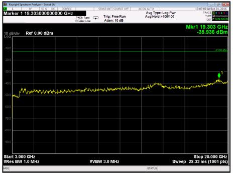
PCS 1900, 1880.0 MHz, 3 GHz to 20 GHz, Spurious Emissions at Antenna Terminals Plot
