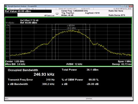
PCS 1900, 1850.2 MHz, Circuit-Switched, 26 dB Bandwidth Plot
