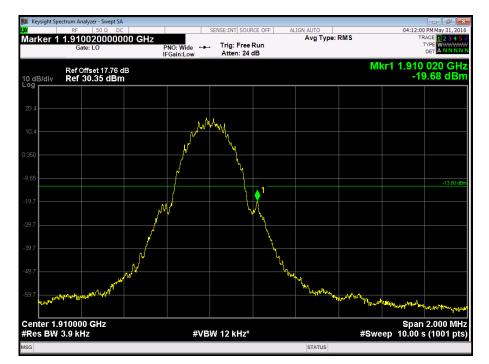
PCS 1900, Circuit-Switched, GMSK, Frequency Block C, Spurious Emissions at Band Edge Plot
