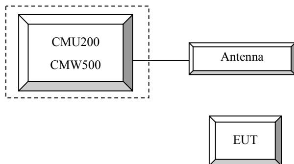
**Block Diagram of Test Setup**
