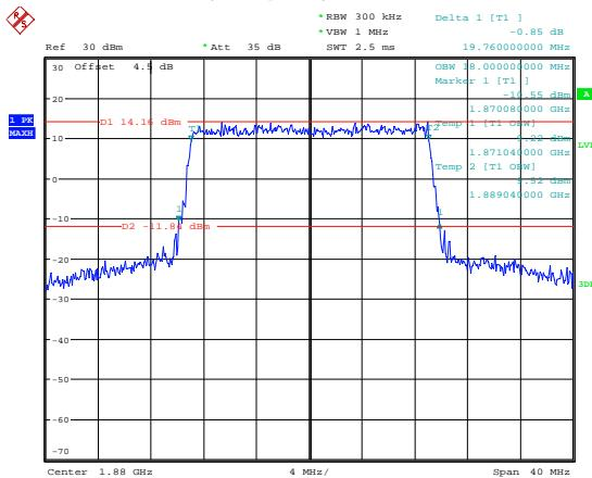
**20M, QPSK, High Channel**
