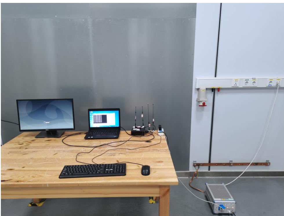
Fig. 4 Power line conducted emission setup photo
