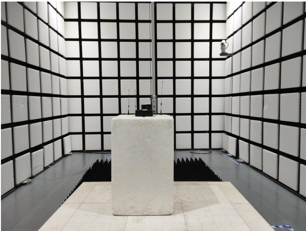
Fig. 3 Radiated emission setup photo(Above 1GHz)
