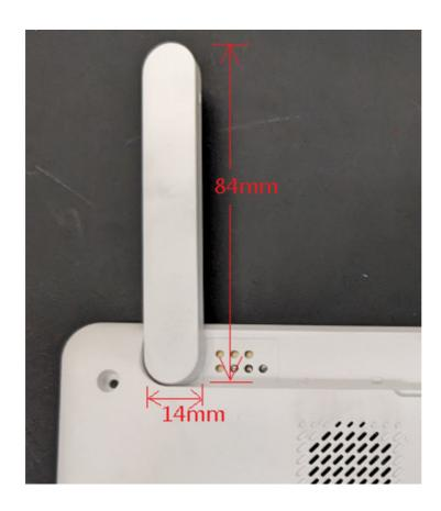
Figure 1 Physical dimension (mm)
