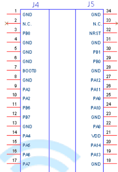
FIGURE 1-2: GL6509 PIN HEADER PIN DIAGRAM(Top View)
