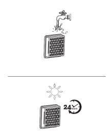
The HEPA filter can be washed under running water and must be completely dry before reinstalling.
