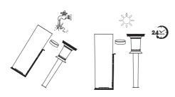
The HEPA mesh filter and dustbin can be washed under cold running water and must be completely dry before reinstalling.
