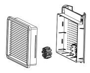
Put the deodorizer into the slot of HEPA cover as shown above.
