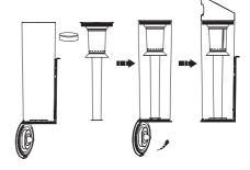
After cleaning, install the HEPA mesh filter dustbin back into the Clean Station.
