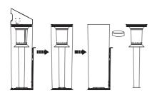
Turn counter-clockwise to open the upper cover, and then remove the filter cotton and filter element.
