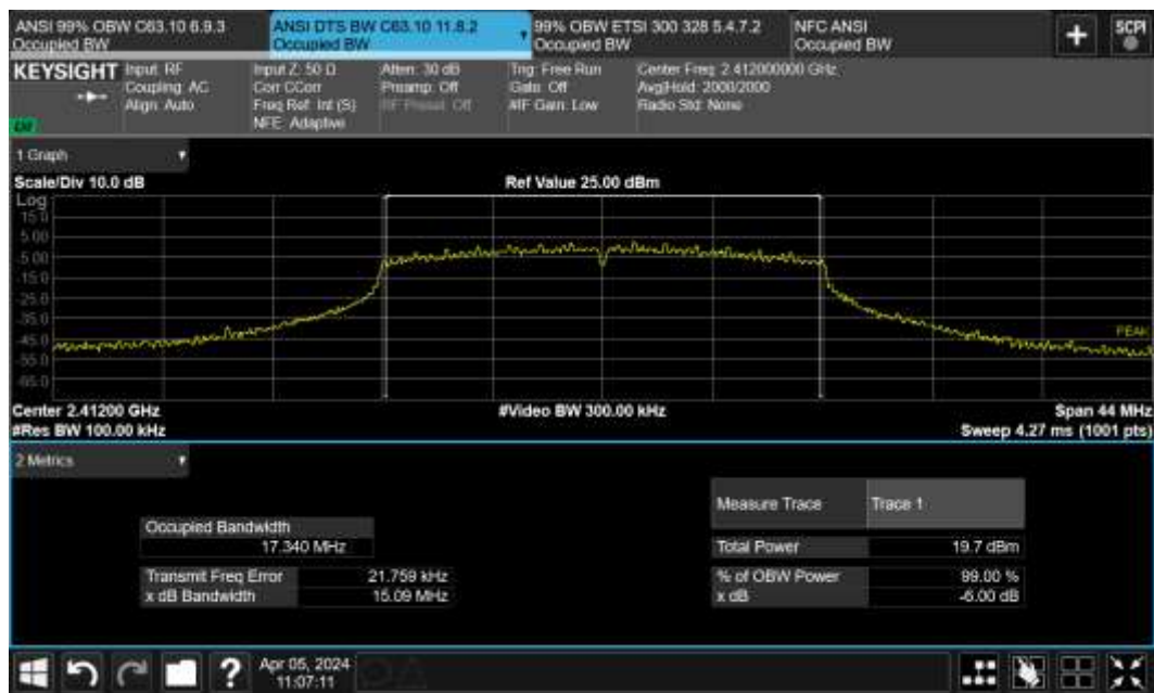
Figure TR06.7: Bandwidth data for 802.11n MCS7 at channel 1
