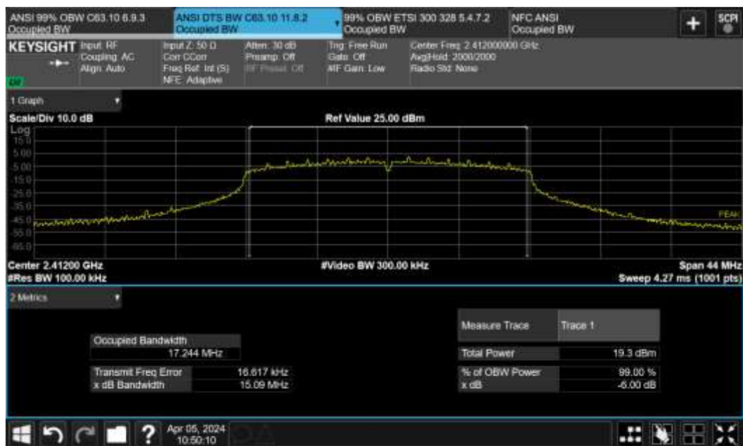
Figure TR06.6: Bandwidth data for 802.11n MCS2 at channel 1
