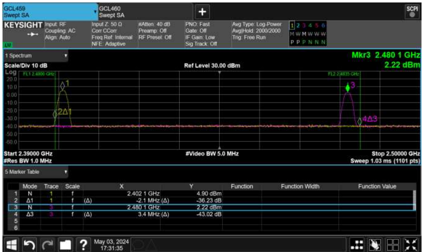
Figure TR43.2: Spectral plot for 36 °C and 5 V test condition
