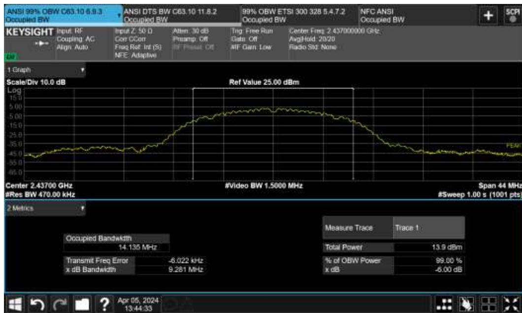
Figure TR10.3: Bandwidth data for B1 Modulation on Channel 6 (2440 MHz)
