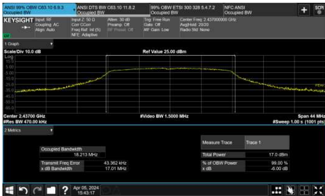
Figure TR10.5: Bandwidth data for NMCS0 Modulation on Channel 6 (2440 MHz)
