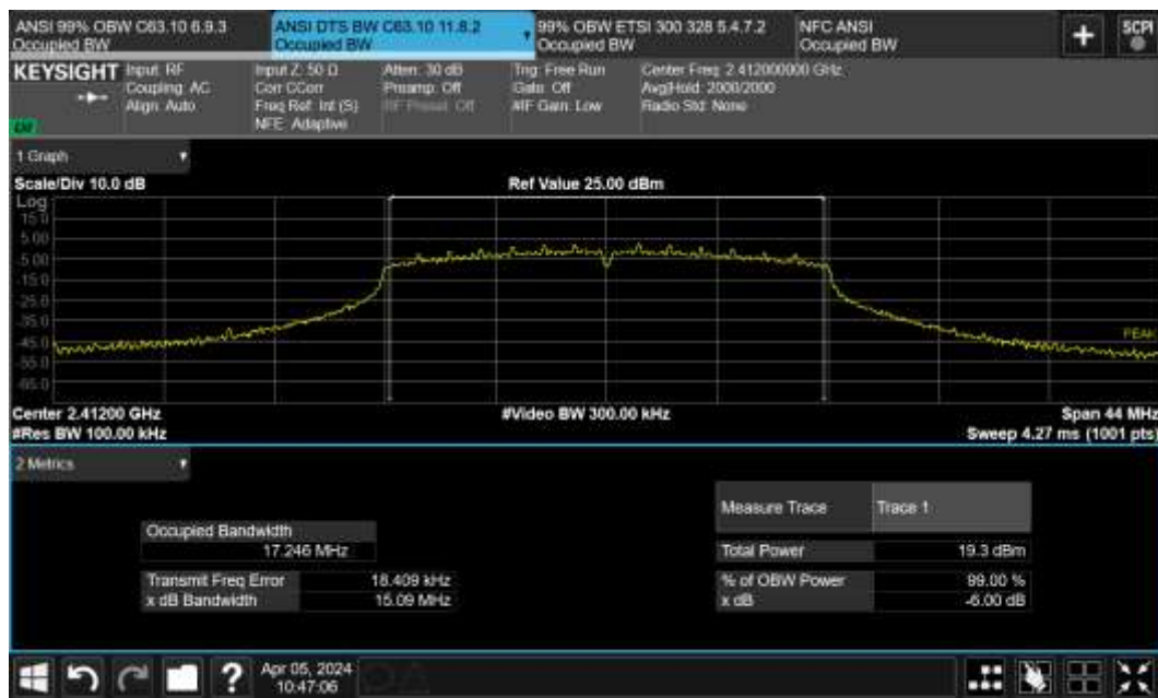
Figure TR06.5: Bandwidth data for 802.11n MCS1 at channel 1
