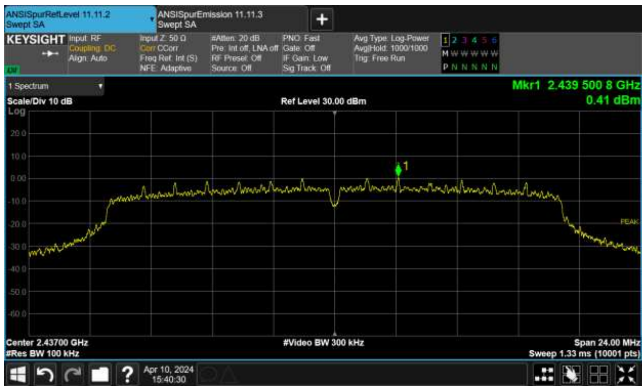
Figure TR27.10: Reference level measurement for IEEE 802.11 N MCS0 on Ch.6
