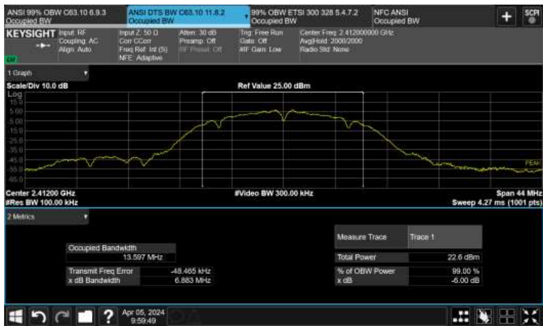
Figure TR06.3: Bandwidth data for 802.11b 2 Mbps at channel 1
