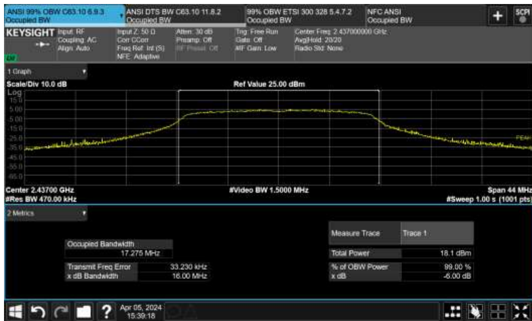
Figure TR10.4: Bandwidth data for G9 Modulation on Channel 6 (2440 MHz)
