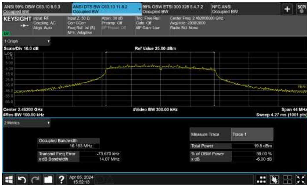
Figure TR06.4: Bandwidth data for 802.11g 6 Mbps at channel 11
