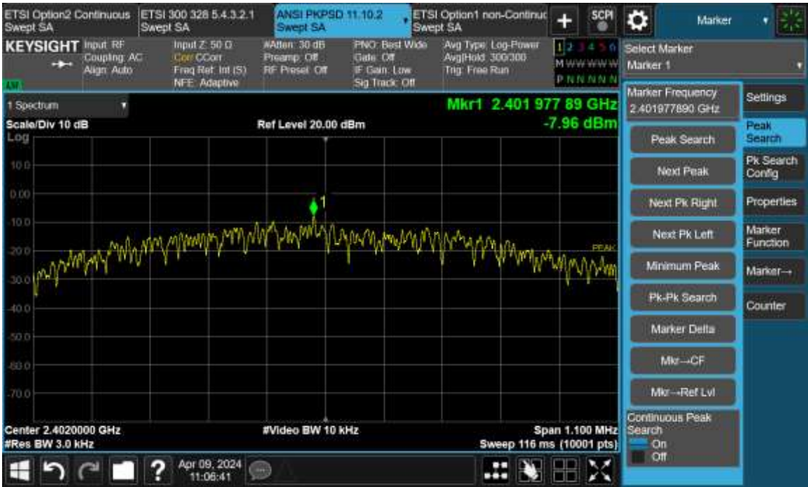
Figure TR19.2: Test data for BLE 1 Mbps, 2402 MHz
