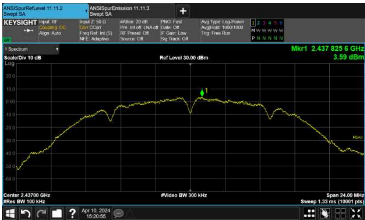
Figure TR27.6: Reference level measurement for IEEE 802.11 B 2 Mbps on Ch.6
