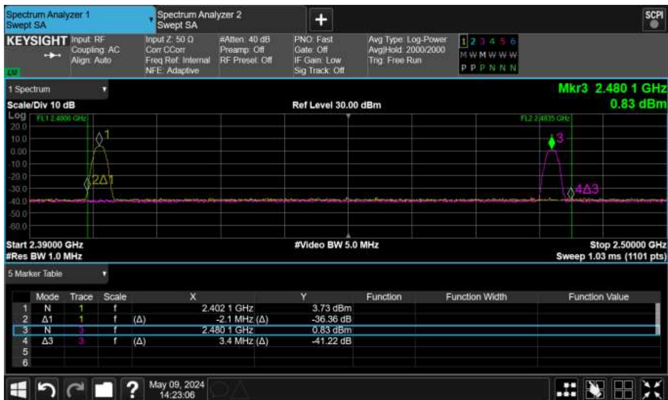
Figure TR43.4: Spectral plot for 20 °C and 4.25 V test condition
