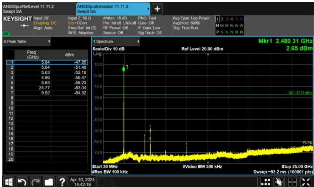
Figure TR27.3 Spectral data for Bluetooth BLE 1 Mbps at 2480 MHz
