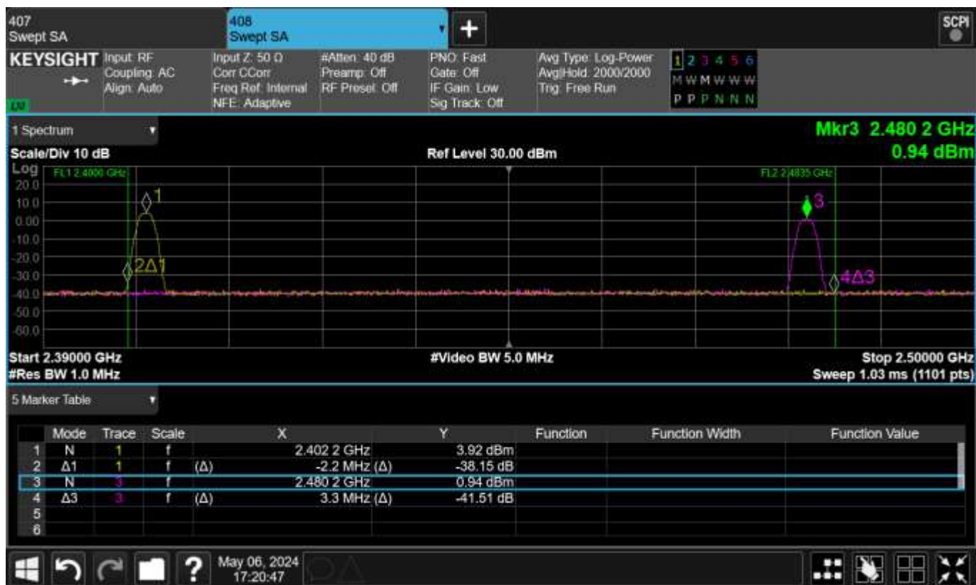
Figure TR43.5: Spectral plot for -20 °C and 5 V test condition
