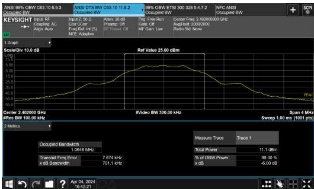
Figure TR06.2: Bandwidth data for BLE 1 at low channel (2402 MHz)
