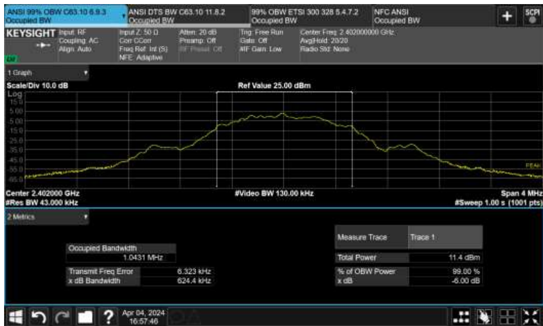
Figure TR10.2: Bandwidth data for BLE 1 Mbps at 2402 MHz
