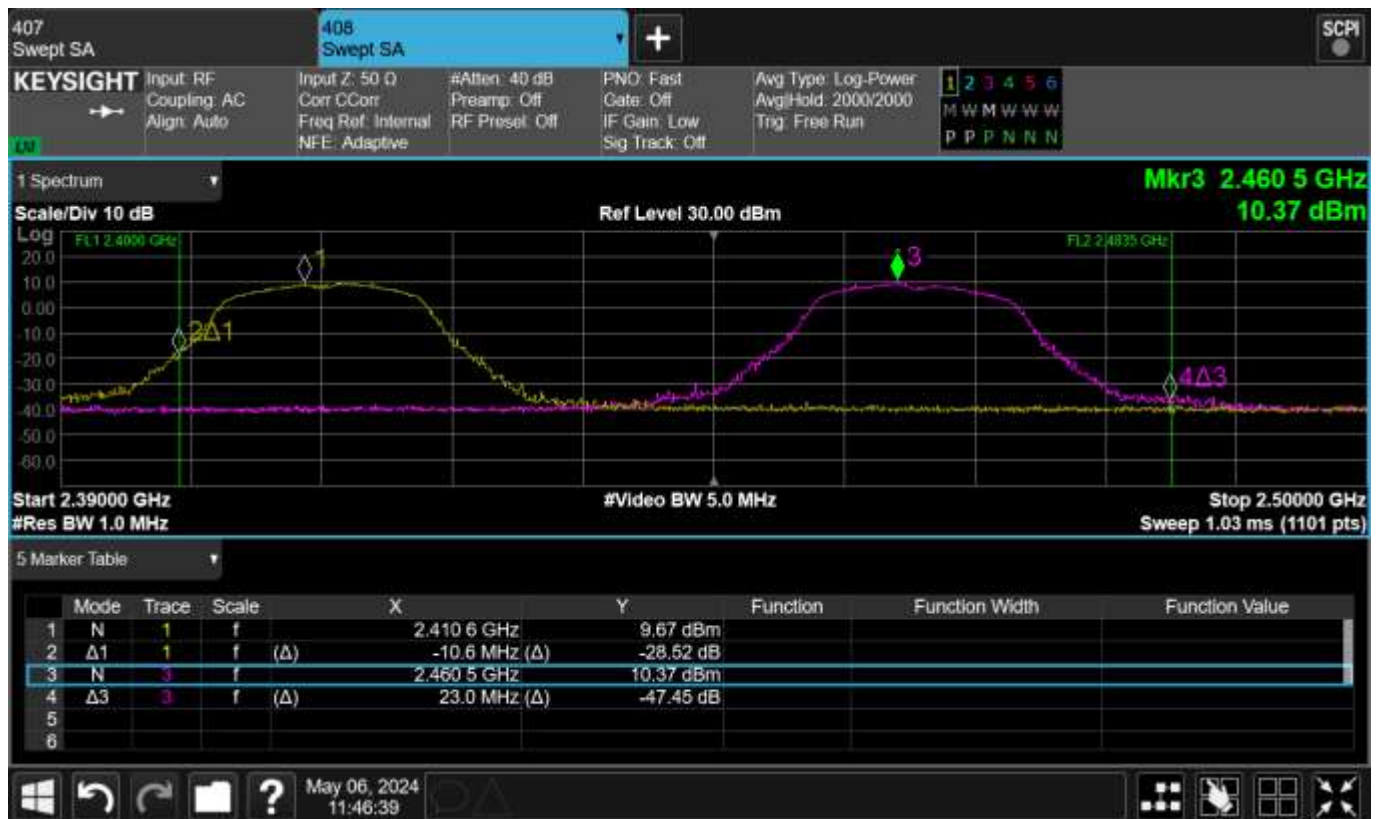
Figure TR44.3: Spectral plot for 20 °C and 5 V test condition
