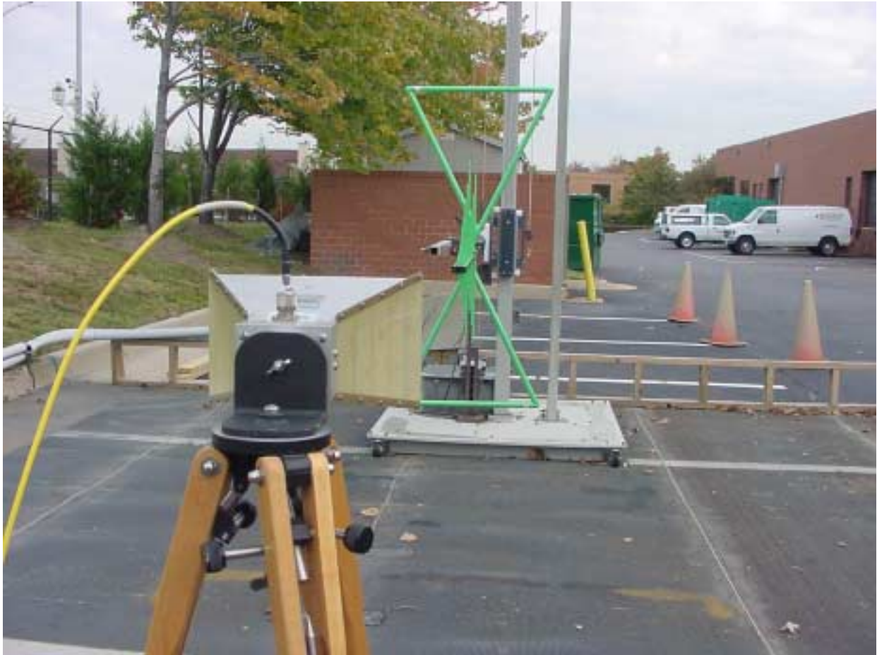
PHOTOGRAPH 5: SUBSTITUTION TRANSMITTING HORN ANTENNA USED FOR FREQUENCIES (1 GHZ-18 GHZ)
