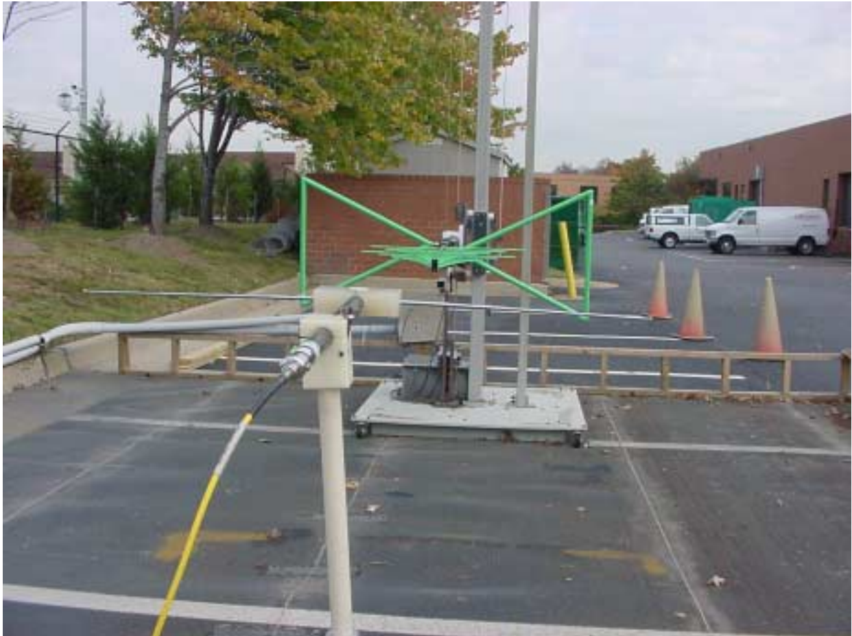
PHOTOGRAPH 4: SUBSTITUTION TRANSMITTING DIPOLE ANTENNA USED FOR FREQUENCIES (30 MHZ – 1 GHZ)
