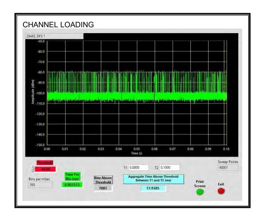
The level of traffic loading on the channel by the EUT is 17.938%
