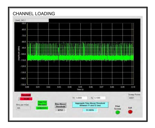
The level of traffic loading on the channel by the EUT is 17.1%
