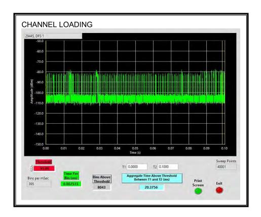
The level of traffic loading on the channel by the EUT is 20.37%
