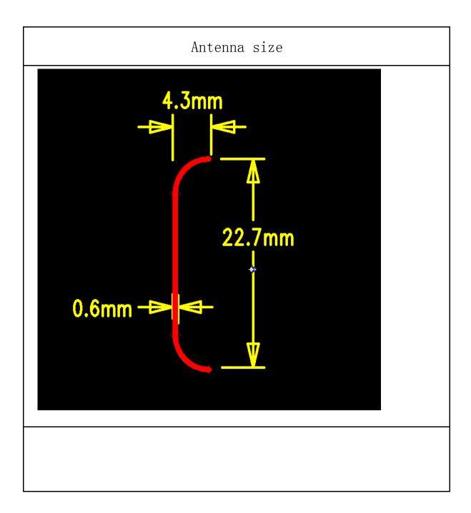
Remote control antenna specification Antenna size:
