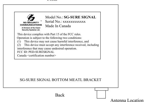
The FCC Label (4.00" x 1.00") is placed on the back of the metal bracket that holds the PCB and the radio modem. Please see attached drawing.
