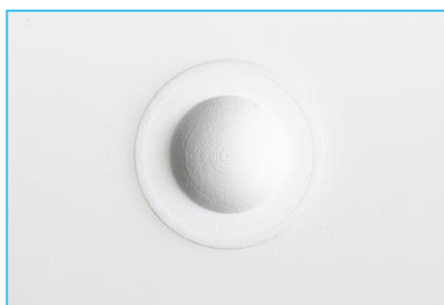
Figure 2.4. HBL lens diameter 36.3 mm and height 9 mm
