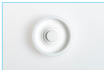
Figure 2.5. FZP lens diameter 36.3 mm and height 7.8 mm
