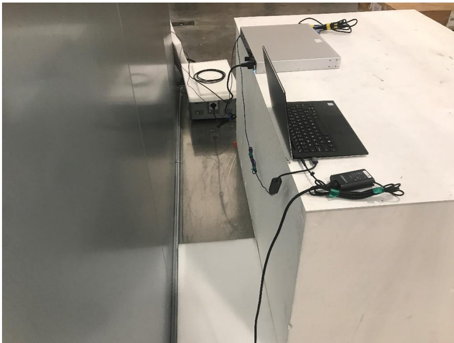
Photograph 6: View Test Set Up Back Conducted Emissions
