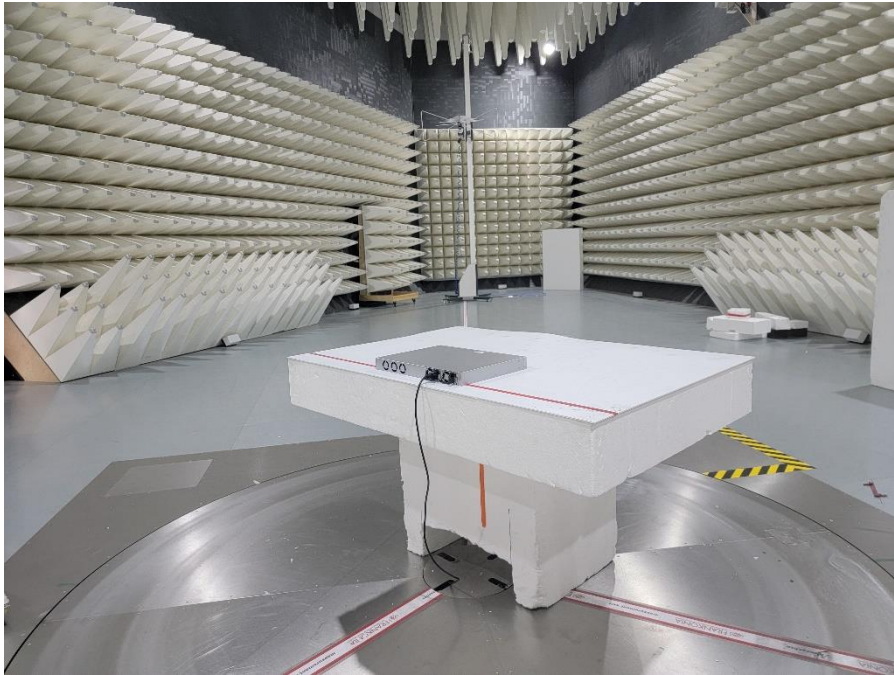
Photograph 1: View Test Set Up Radiated Emissions 30 – 1000 MHz
