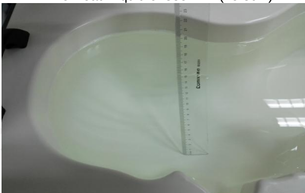
The Head Liquid of 1800MHz (15.2cm)
