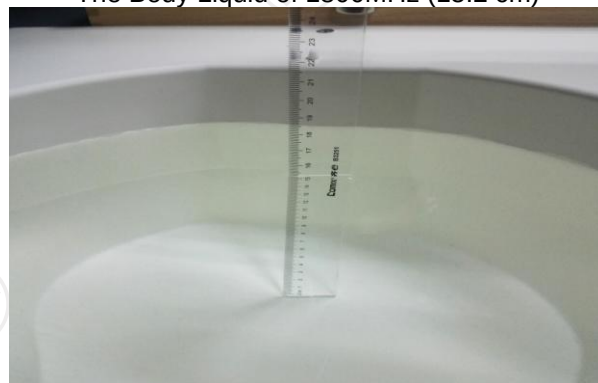
The Body Liquid of 2450MHz (15.3cm)
