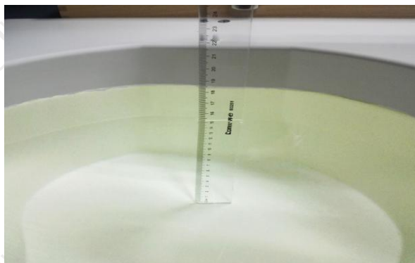
The Body Liquid of 1800MHz (15.2 cm)
