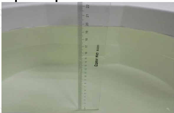
The Body Liquid of 835MHz (15.4cm)
