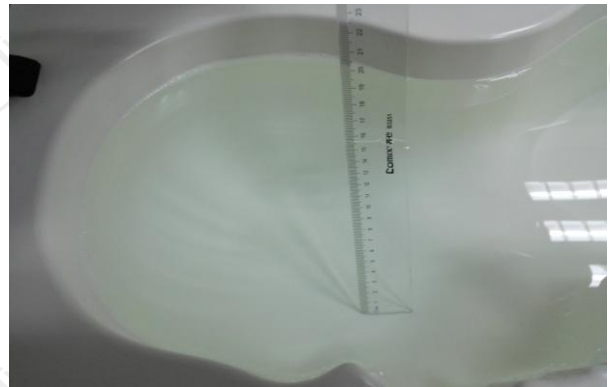
The Head Liquid of 2450MHz (15.6cm)
