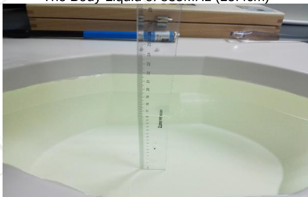
The Body Liquid of 1900MHz (16.4 cm)
