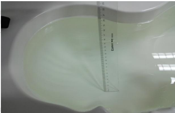
The Head Liquid of 1900MHz (15.5cm)
