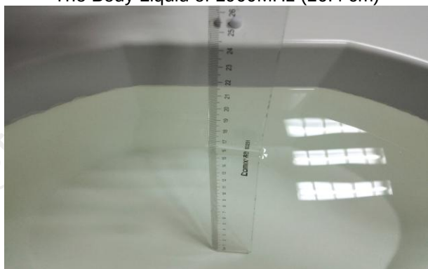
The Body Liquid of 2600MHz (16.5cm)
