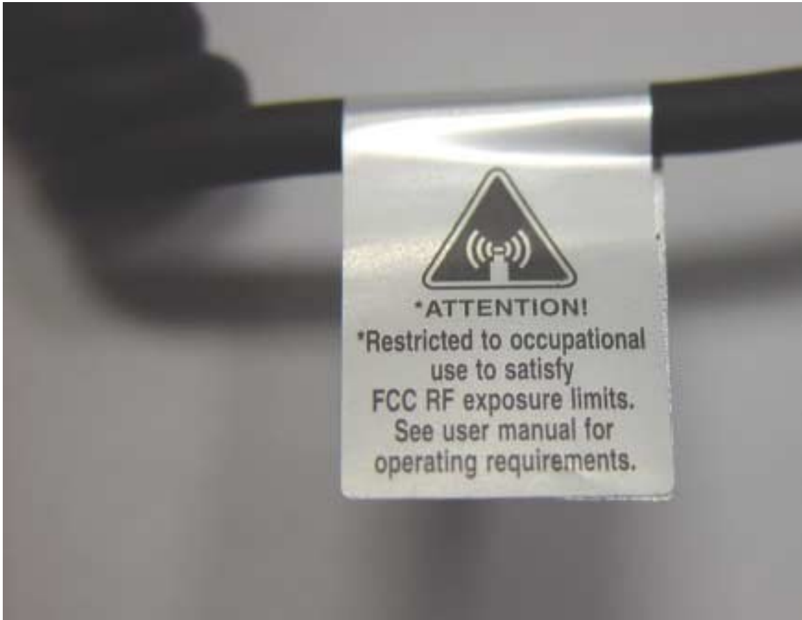
CLOSE-UP VIEW OF RF SAFETY LABEL ON MICROPHONE CORD
