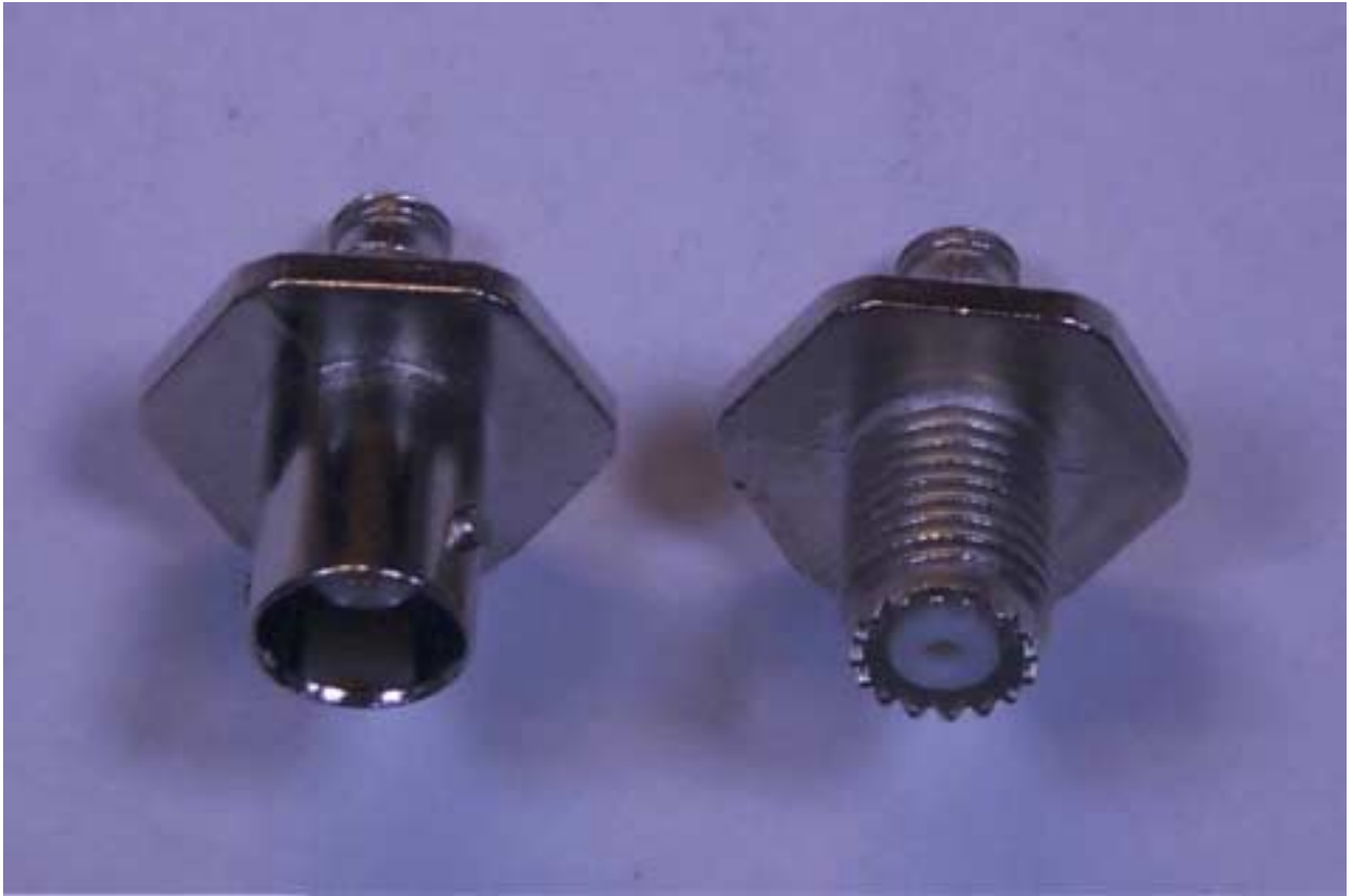
CLOSE-UP VIEWS OF BNC (LEFT) AND MINI-UHF (RIGHT) ANTENNA CONNECTORS
