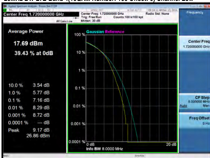
20MHz BW LTE-Band 4(16QAM Number: 100 Offset: 0) Channel Mid
