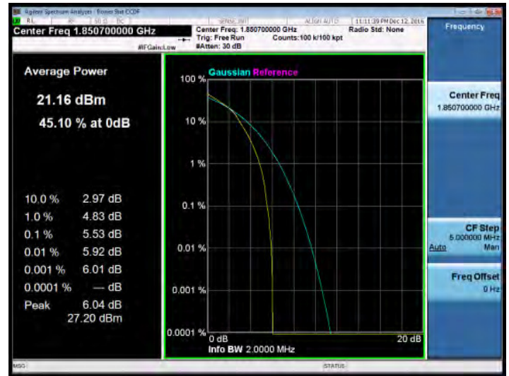
1.4MHz BW LTE-Band 2(16QAM Number: 6 Offset: 0) Channel Mid
