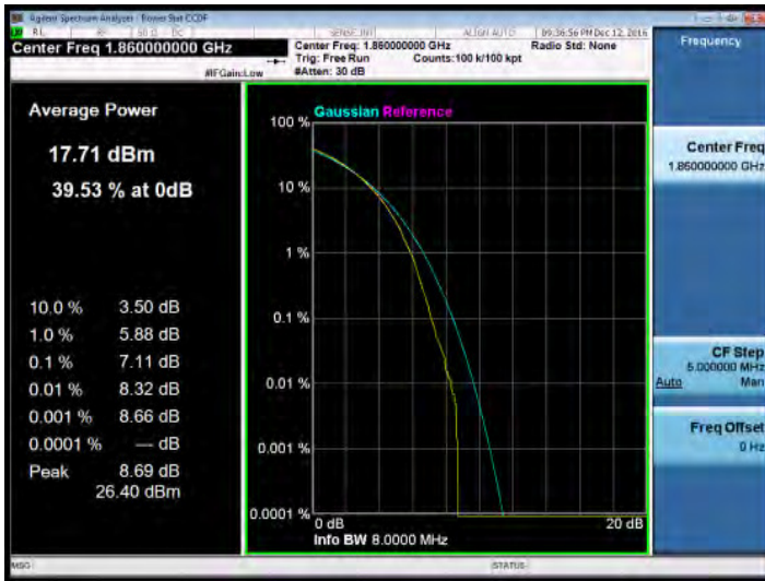
20MHz BW LTE-Band 2(16QAM Number: 100 Offset: 0) Channel Mid
