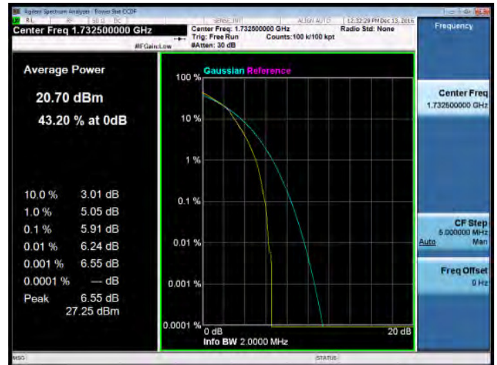
1.4MHz BW LTE-Band 4(16QAM Number: 6 Offset: 0) Channel High
