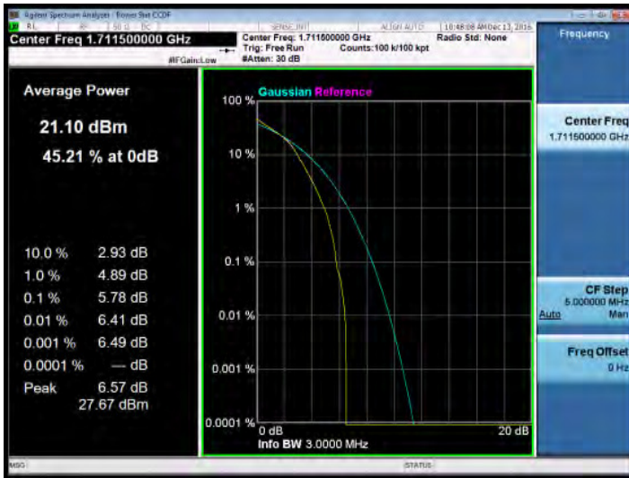
3MHz BW LTE-Band 4(16QAM Number: 15 Offset: 0) Channel Mid
