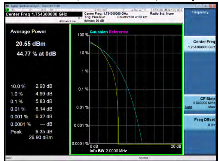
1.4MHz BW LTE-Band 4(16QAM Number: 6 Offset: 0) Channel High
