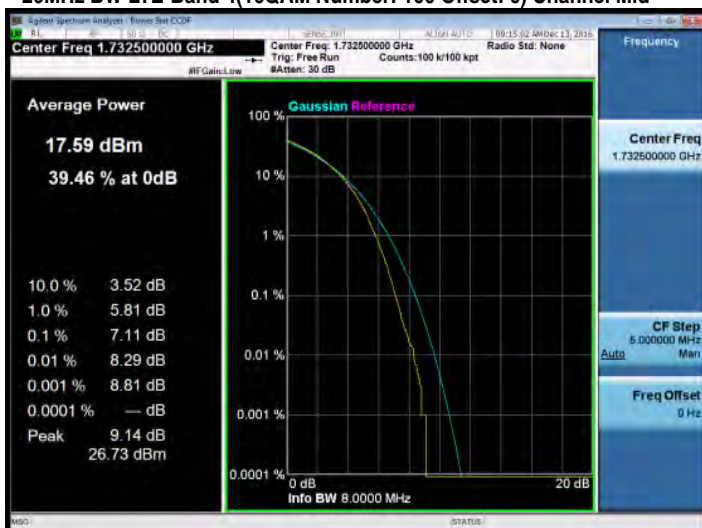
20MHz BW LTE-Band 4(16QAM Number: 100 Offset: 0) Channel Mid
