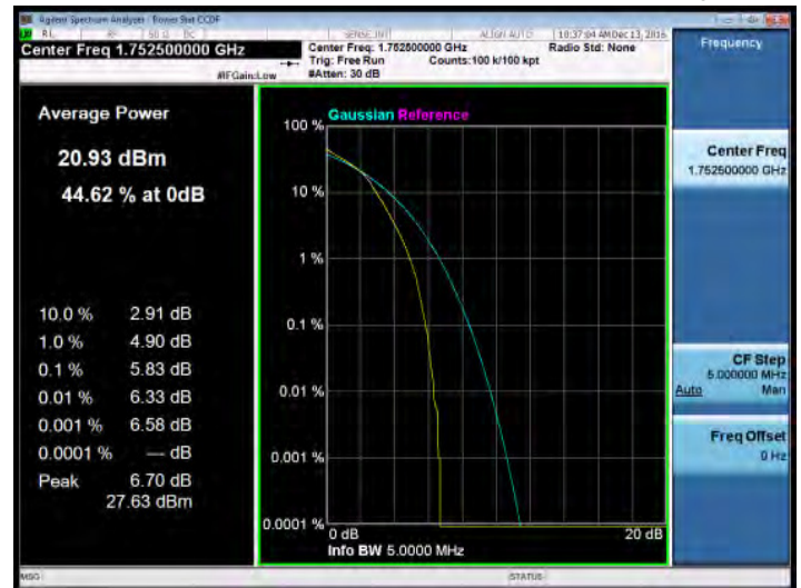
5MHz BW LTE-Band 4(16QAM Number: 25 Offset: 0) Channel High
