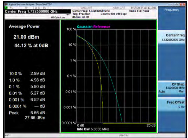
5MHz BW LTE-Band 4(16QAM Number: 25 Offset: 0) Channel High
