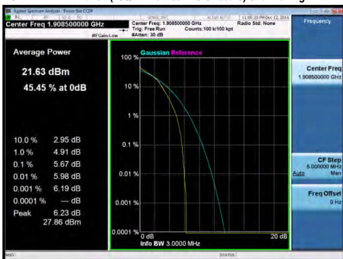
3MHz BW LTE-Band 2(16QAM Number: 15 Offset: 0) Channel High
