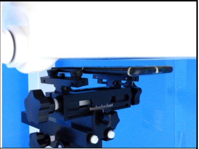
Front Face of EUT with 1.0 cm Gap
