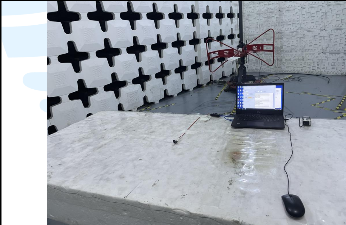
Radiated emission Test Setup (30 MHz~1 GHz)_ Right Ear
