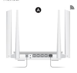
A Wi-Fi: Connect your device to the router's Wi-Fi using the SSID (network name) and Password printed on the bottom of the router.
