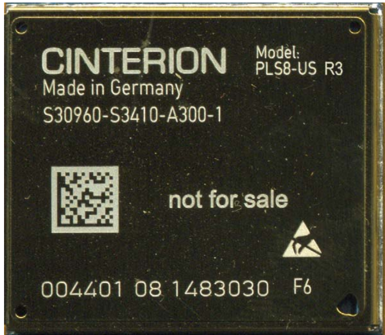
PLS8-US R3 label location lasing on shielding
