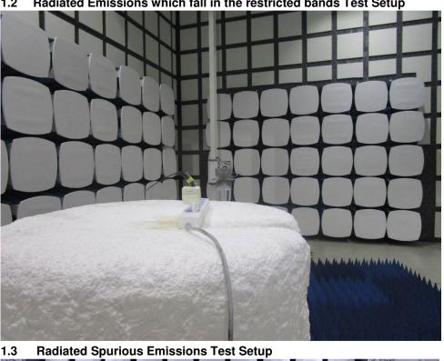
1.2 Radiated Emissions which fall in the restricted bands Test Setup
