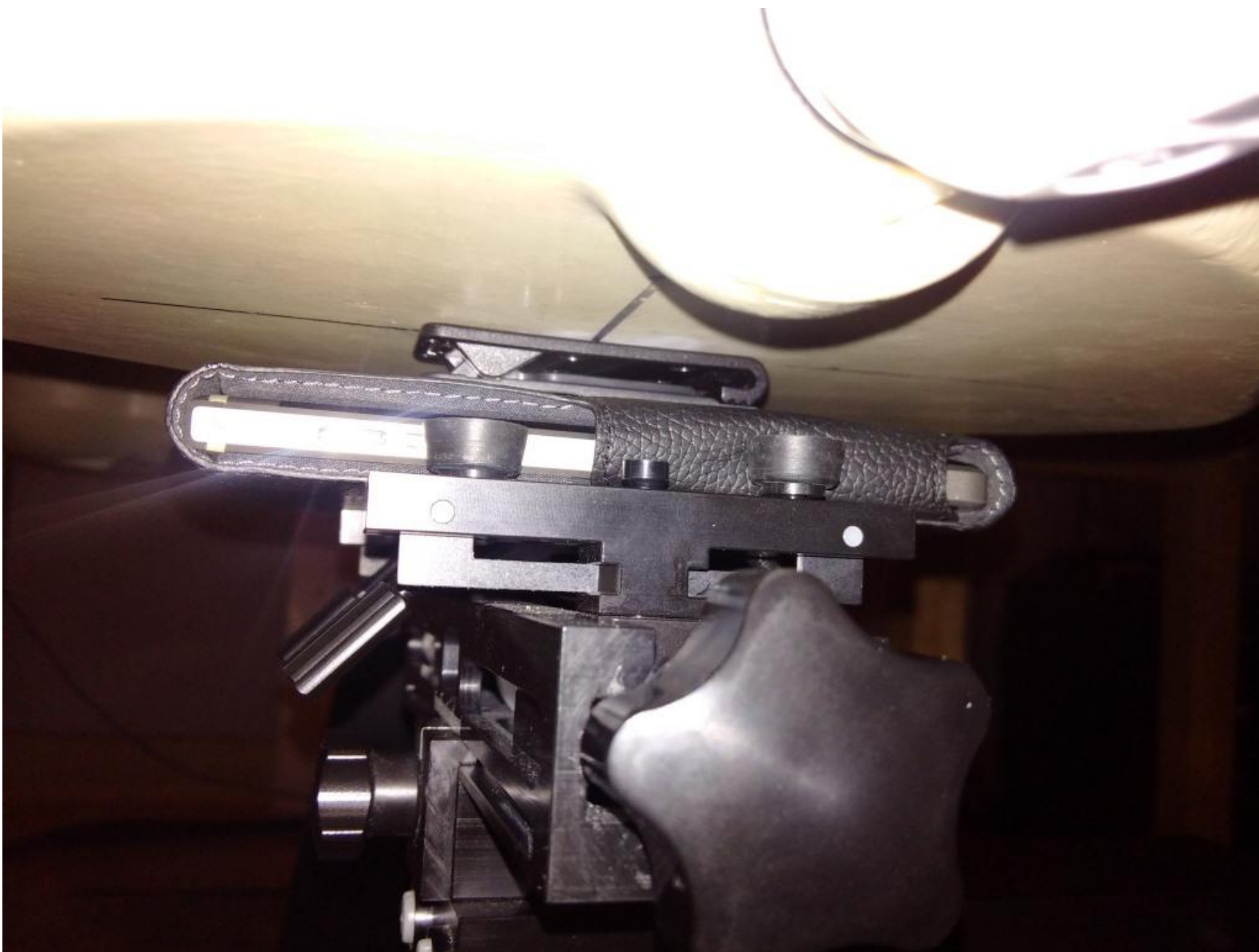
Figure E15. Body-worn configuration (Holster, back)
