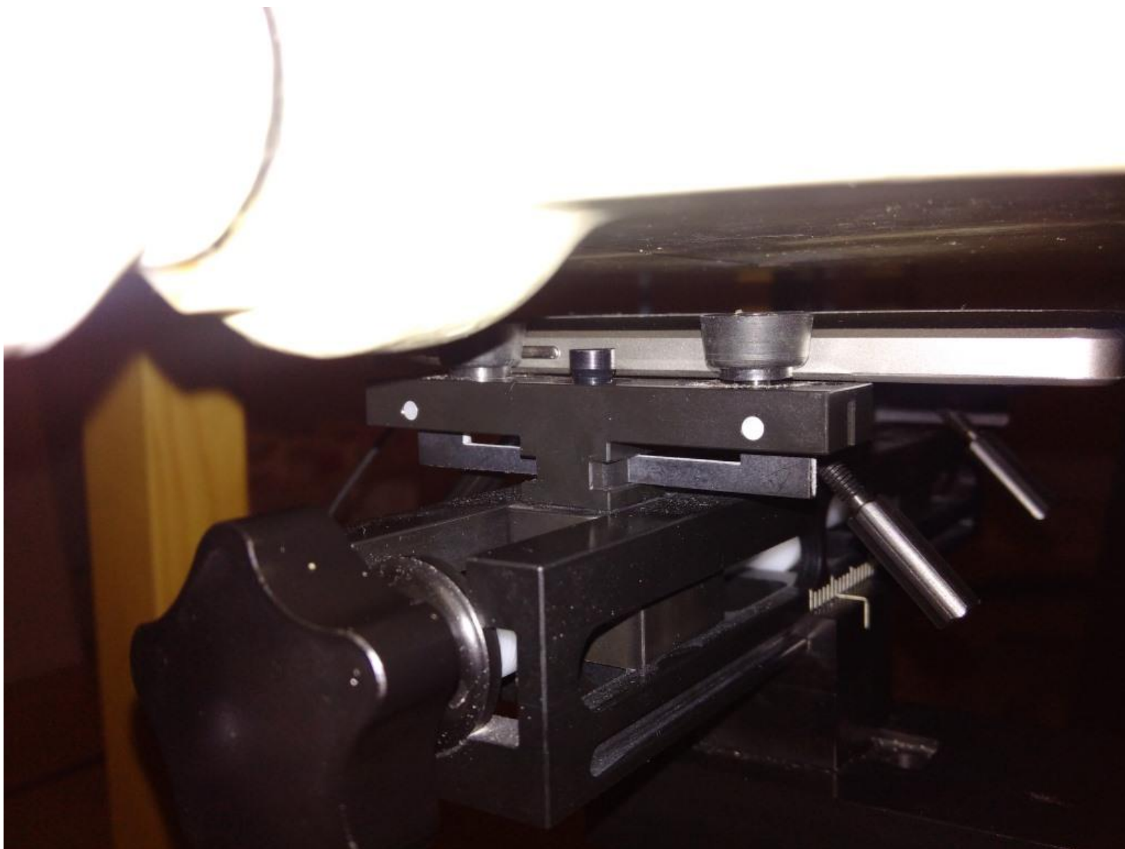
Figure E12. Hotspot configuration (No Holster, Headset, back side 10mm away)
