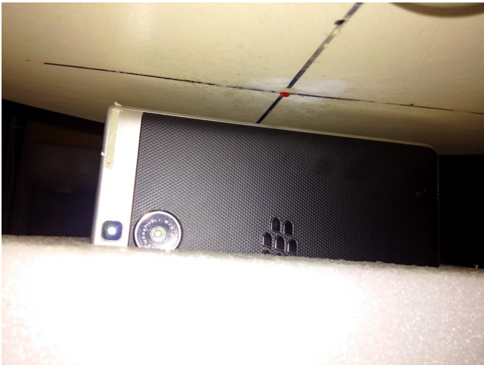
Figure E8. Hotspot configuration (No Holster, left side 10mm away)
