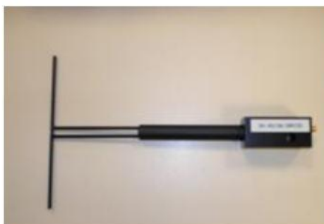
Figure 1 – Satimo COMOSAR Validation Dipole
