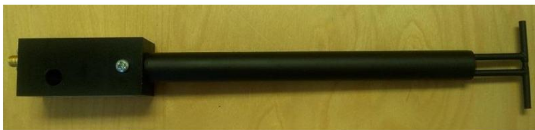
Figure 1 – MVG COMOSAR Validation Dipole
