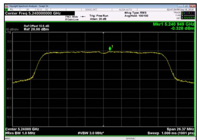
U-NII-1 Power spectral density-802.11 n(20MHz),5240MHz,Ant1
