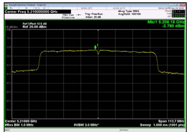
U-NII-1 Power spectral density-802.11 ac(80MHz),5210MHz,Ant1
