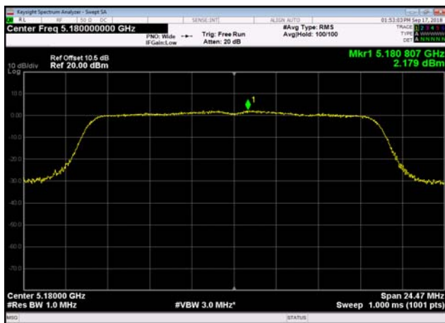
U-NII-1 Power spectral density-802.11 a(20MHz),5180MHz,Ant0
