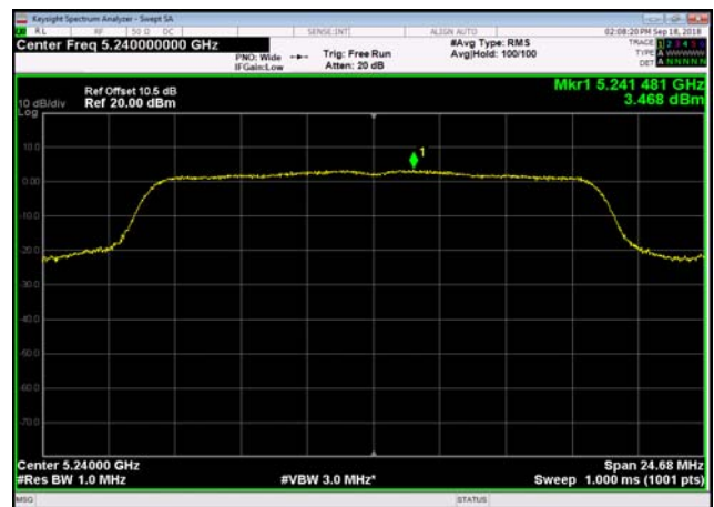
U-NII-1 Power spectral density-802.11 ac(20MHz),5180MHz,Ant1
