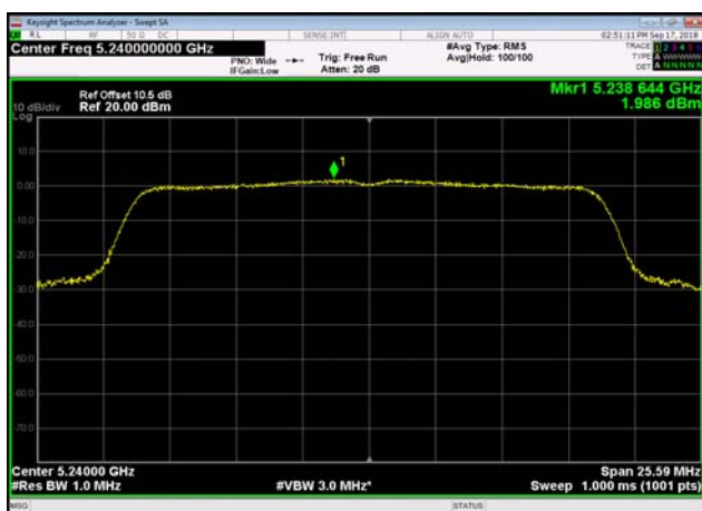
U-NII-1 Power spectral density-802.11 n(20MHz),5240MHz,Ant0
