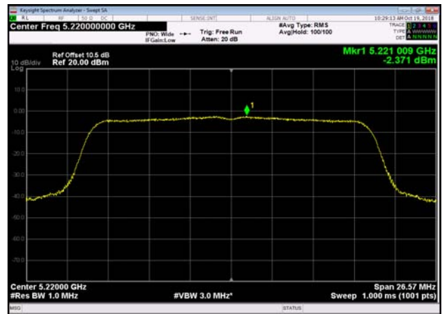
U-NII-1 Power spectral density-802.11 ac(20MHz),5240MHz,Ant1
