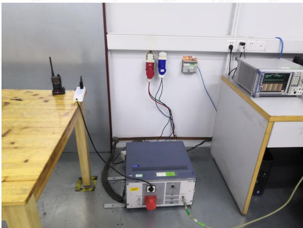
RADIATED EMISSION TEST SETUP-BELOW 1GHZ
