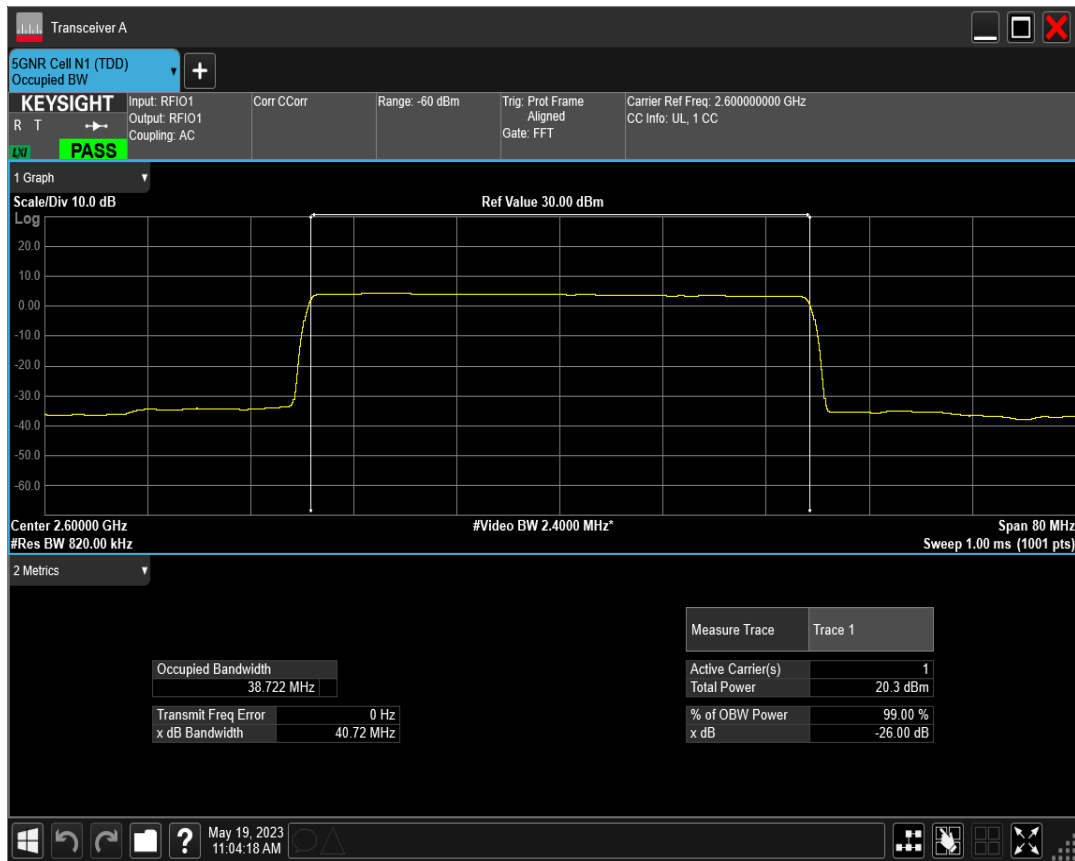
n38 SCS=15kHz DFT_QAM256 BW=40MHz Channel=520000 RB=216@0
