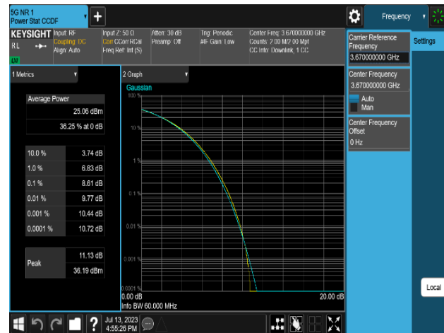
Plot 8-40. Peak To Average Power Ratio Plot (n48_3C_20M+20M+20M_16QAM - High Channel_8T, Port 2)
