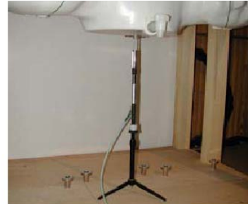
Figure 9.1 Dipole Verification Test Setup Diagram & Photo
