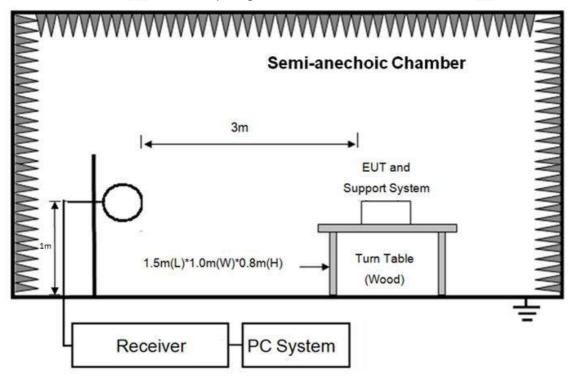
In 3 m Anechoic Chamber, test setup diagram for below 1 GHz
