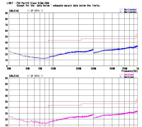
CHART: WITH FACTOR ANT TYPE: -30MHz LOOP, 30-300MHz BICONICAL, 300MHz-1000MHz LOGPERIODIC, 1000MHz HORN CALCULATION: READING + ANT FACTOR + LOSS (CABLE+ATTEN.) - AMP. GAIN Page:
