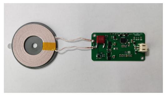
PCB and coil can be unfolded or folded. In order to provide better heat dissipation performance, coil and PCB surface should be separated by more than 3mm when folded.
