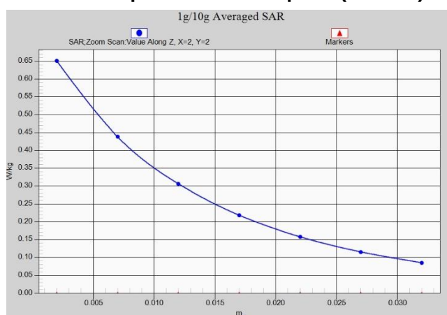
Z-Scan at power reference point (LTEB41)
