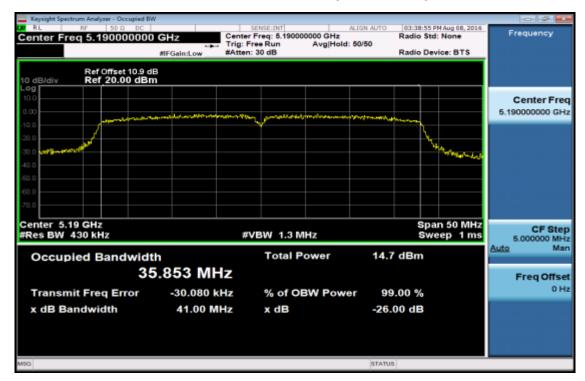
26dB & 99% Band Width Test Data CH-High (5230 MHz)
