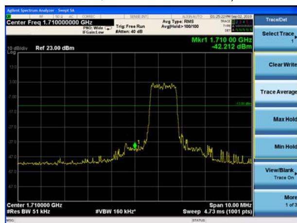
LTE Band 66 QPSK 15MHz CH-Low, 1 RB
