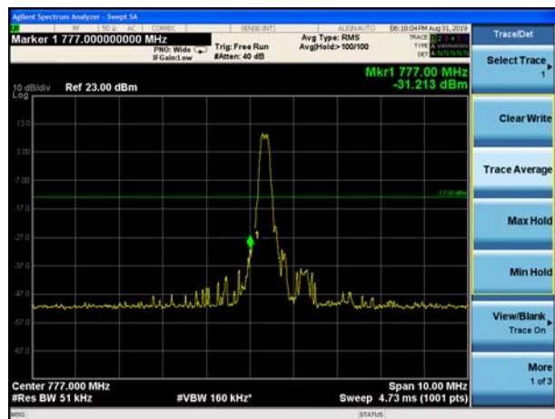
LTE Band 13 QPSK 5MHz CH-Low, 100%RB
