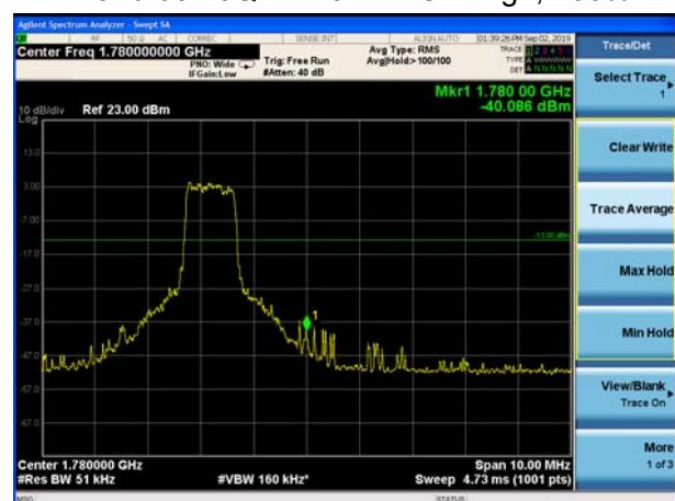
LTE Band 66 16QAM 20MHz CH-High, 100%RB
