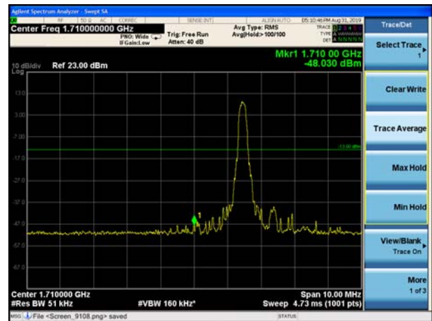
LTE Band 4 16QAM 20MHz CH-High, 100%RB
