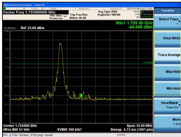
LTE Band 4 16QAM 20MHz CH-Low, 100%RB
