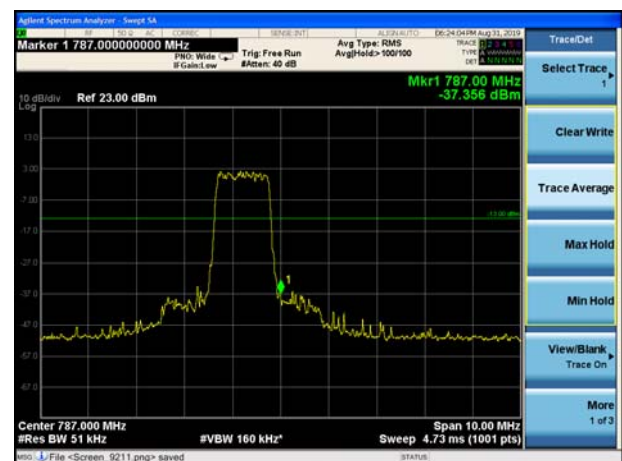
LTE Band 13 QPSK 5MHz CH-High, 100%RB
