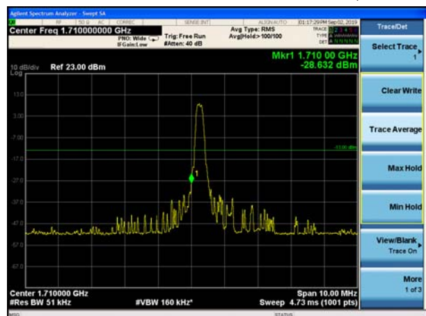
LTE Band 66 16QAM 1.4MHz CH-Low, 100%RB
