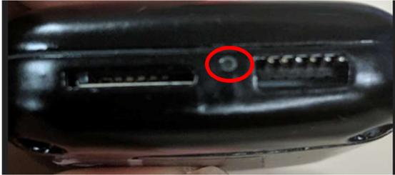
3. Wait a few seconds until the solid yellow light on the BTG25 changes to a blinking yellow light. The blinking yellow light means that the BTG25 has been un-provisioned from the previous device and is ready to be paired to a new device.
