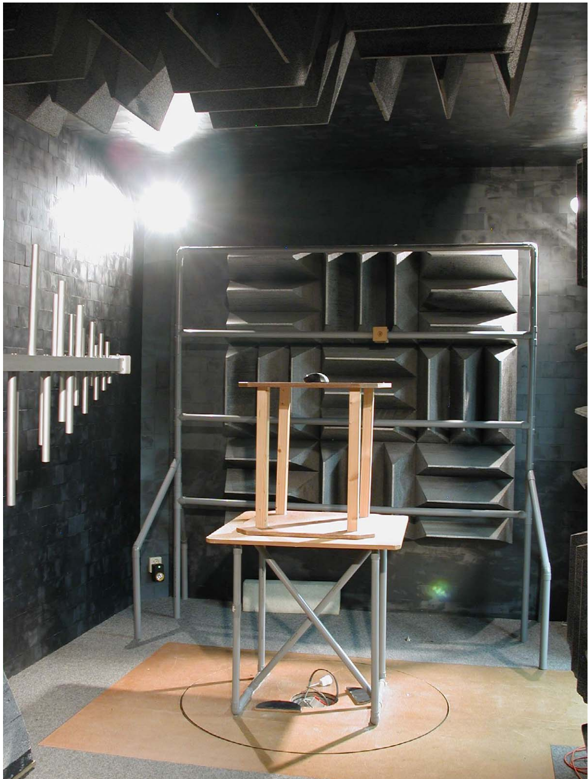
Photograph 1: Test setup 30 - 1000 MHz (exploratory measurements)
