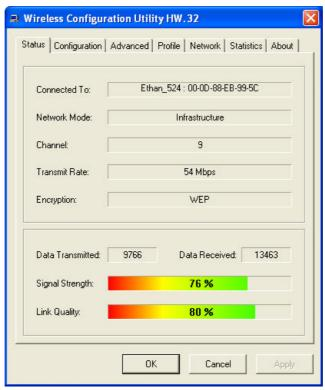
There are two dialog boxes showing the data transmitted and the data received. The two signal lines show the Signal Strength and the Link Quality of the device.
