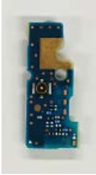
Internal Main_ANT-2-PWB (Front-side)
