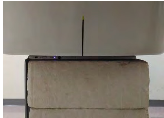
Fig.3 EUT Back side to flat phantom (Laptop mode)
