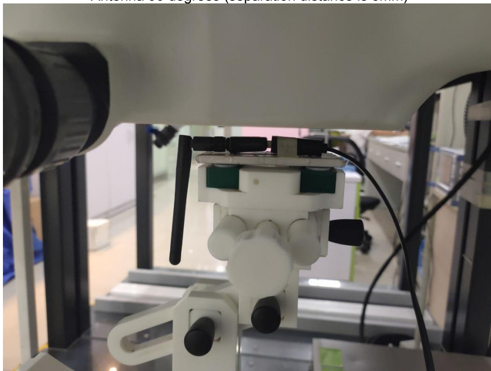
Horizontal- Up Antenna 90 degrees (separation distance is 5mm)
