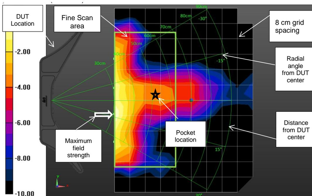
Figure 14: Explanatory Diagram of the X-Y Plane Field Plots
