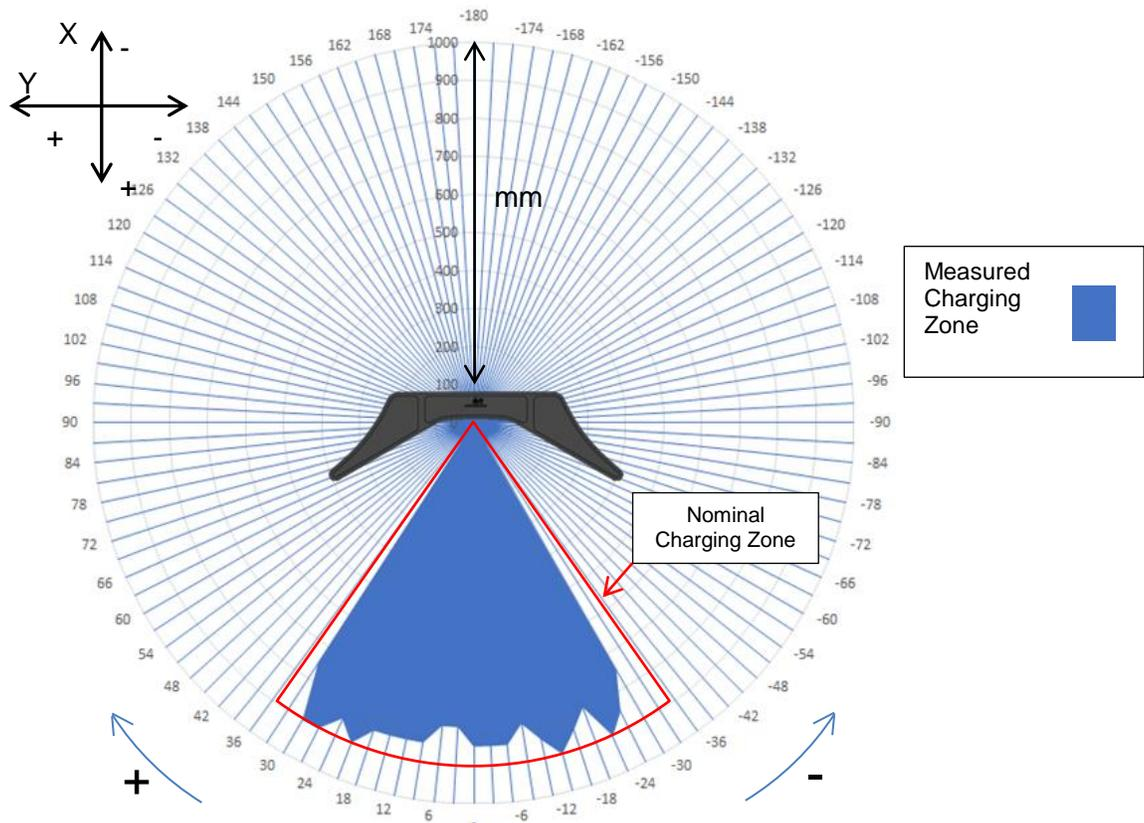
Figure 4: Charging Zone Test Result – X-Y plane
