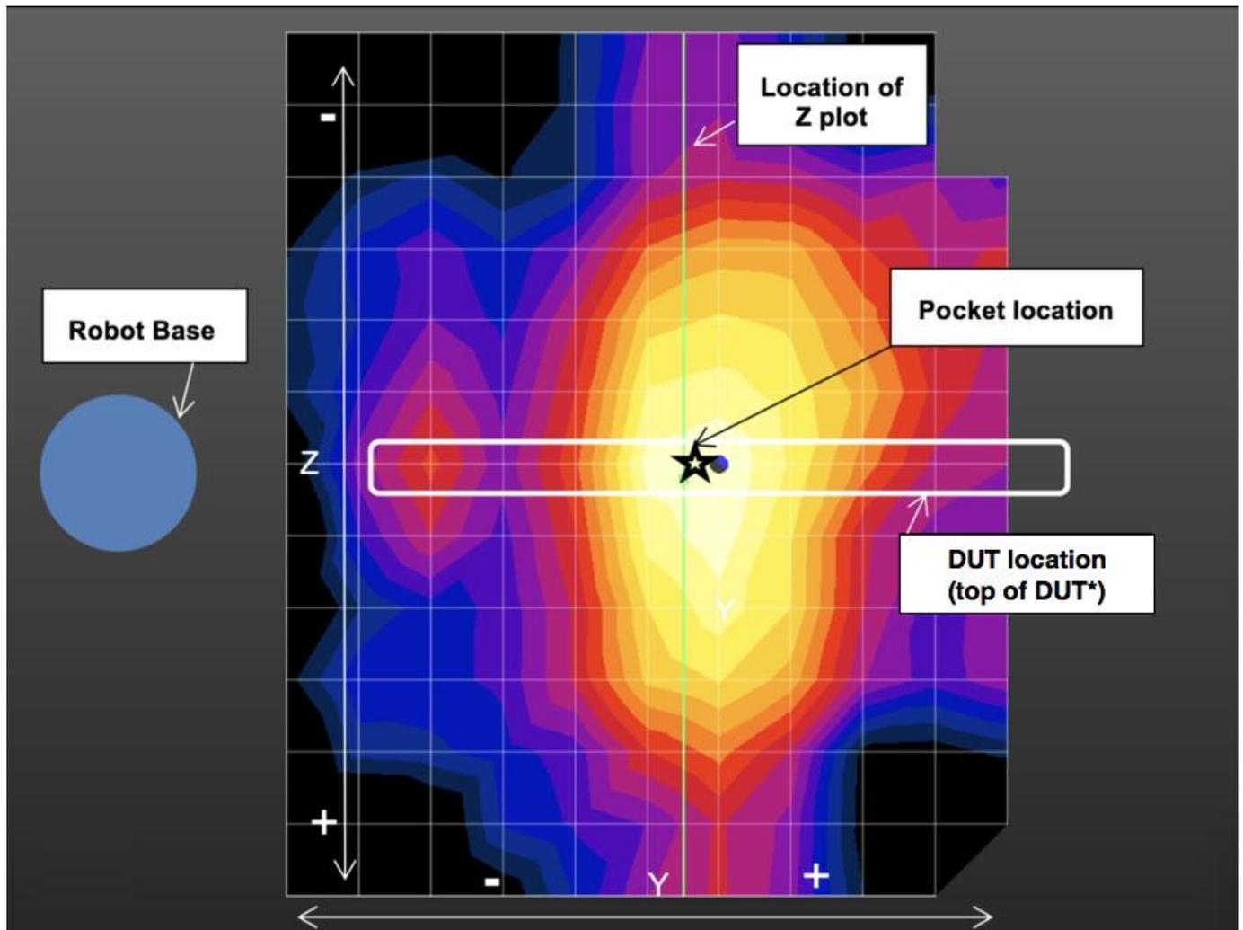
Figure 19: Explanatory Diagram of the Y-Z Plane Field Plots
