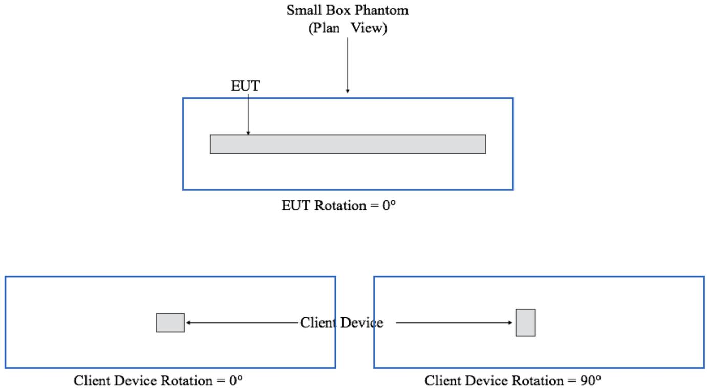
Figure 22: Orientation of DUT and Client Device with Respect to the Phantom
