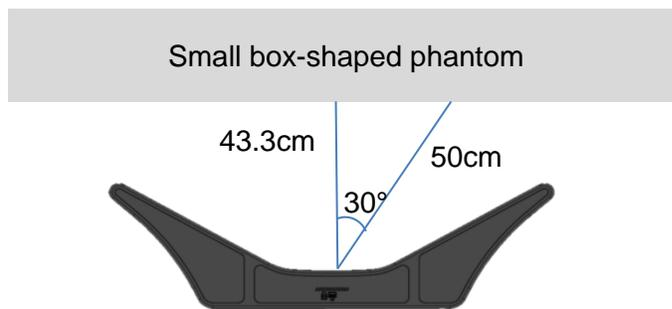
Figure 23: Example of DUT distance from the Phantom
