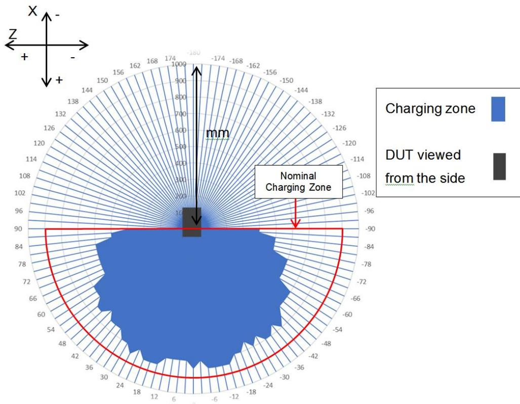
**Figure 5: Charging Zone Test Result – X-Z plane**
