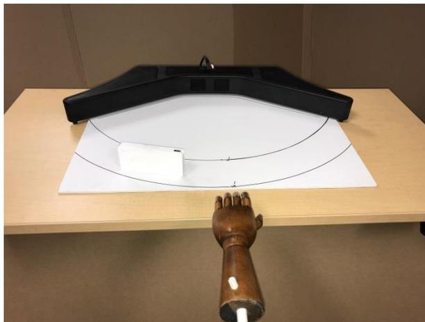
Figure 8: Test setup for Keep-Out Zone Verification.
