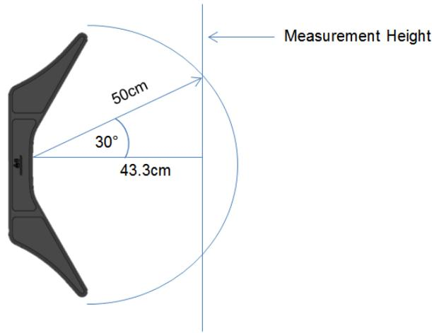
Figure 17: Radial distance versus measurement height
