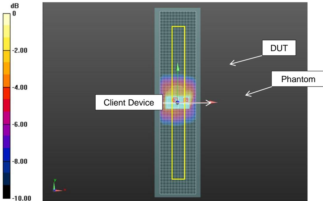
Figure 24: Explanatory Diagram of the SAR plots
