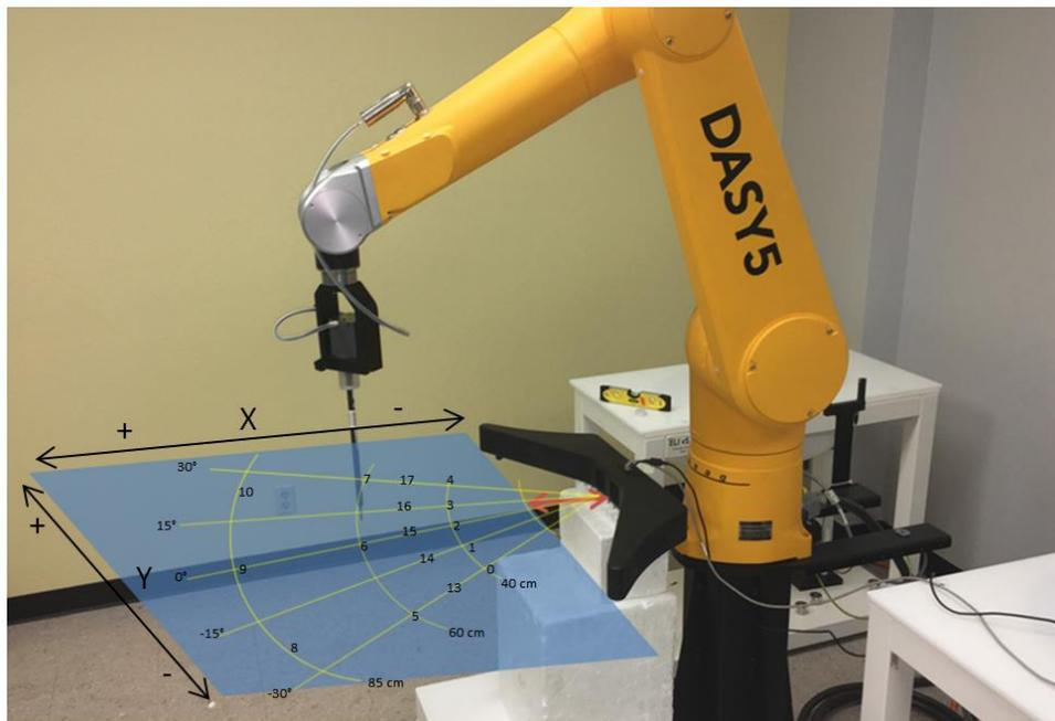
Figure 13: X-Y Plane Field Measurements Test Setup
