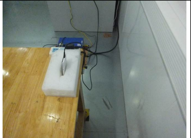
Conducted Emissions Test Setup Side View
