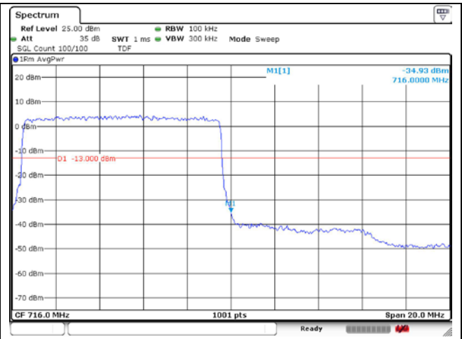
QPSK High Channel - Full RB
