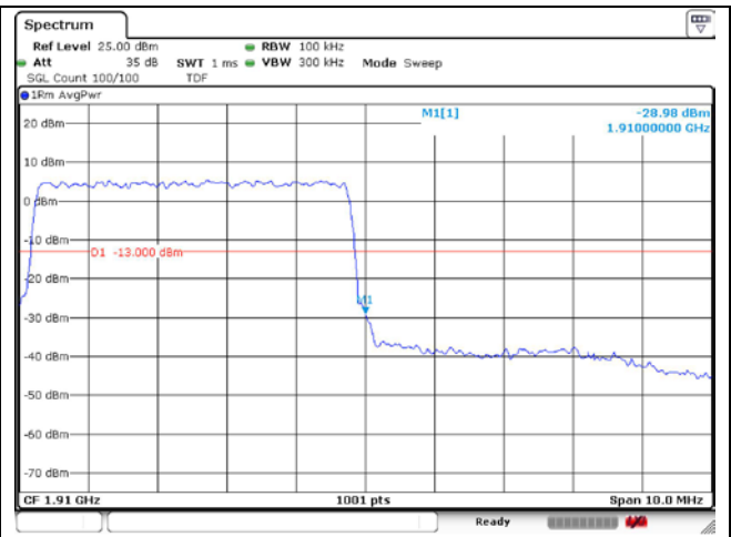
QPSK High Channel - Full RB
