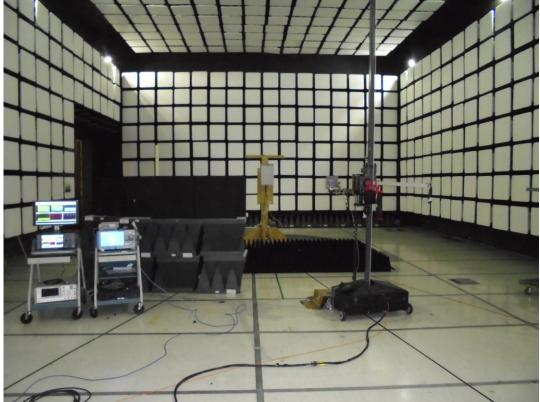
Radiated Spurious Setup for 40-200 GHz
