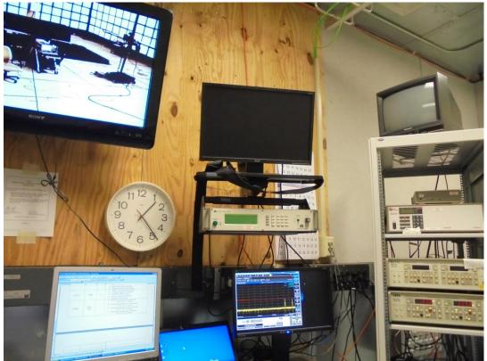
Radiated Setup for Channel Power, Occupied Bandwidth, Edge of band and Modulation.
