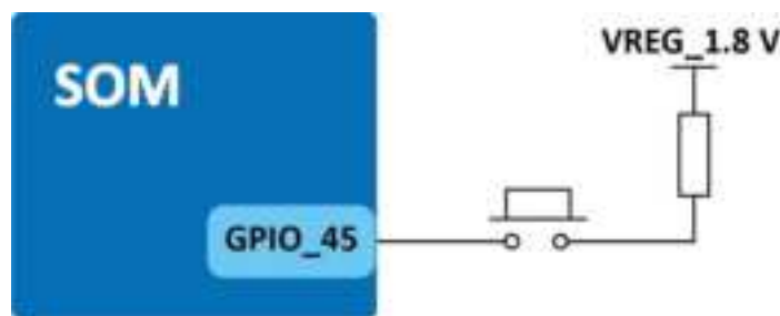
Figure 2-4. Power on Signal
