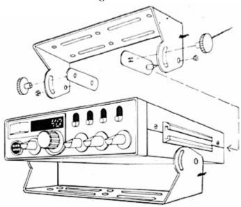
Step 1: Heeding the caution, use the mounting bracket as a template for marking the location of screw holes under the dash. Use an awl, nail or other sharp pointed object to mark the hole locations.
