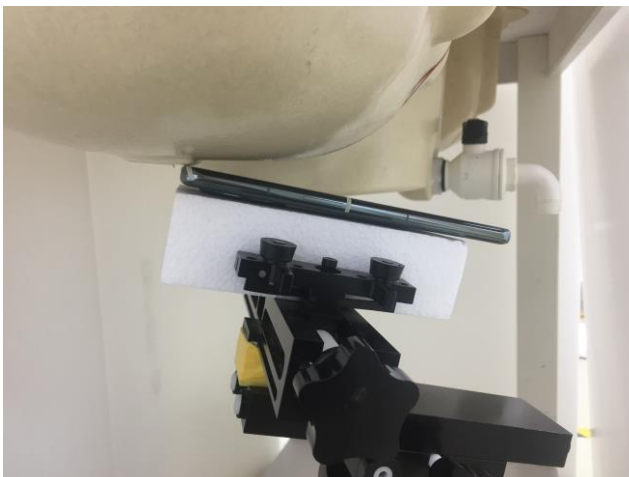
Right Tilted, Test Separation 0 mm
