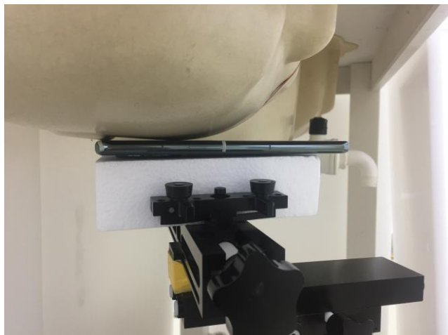
Right Cheek, Test Separation 0 mm
